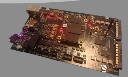
The USI01 board measuring 160 x 100 mm and weighs 127 grams
